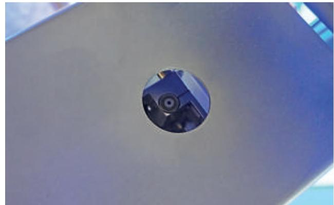
*micro drop jet fluxer: highly precise and minimum consumption*
