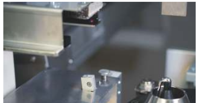
precise micro drop jet fluxer with automatic function and position control
