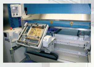
In height adjustable work place with swiveling table for ergonomical assembly and repair of boards. The unit is equipped with a dual conveyor and cross transfer.
